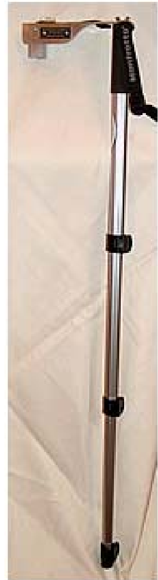
Figure 1. Laser point sampler for line-point intercept (photo courtesy J. Alexander).
